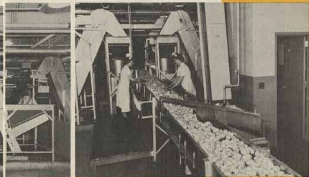
Four bucket conveyors raise the processed potatoes on their "elevator ride" to the production room floor above . . .
